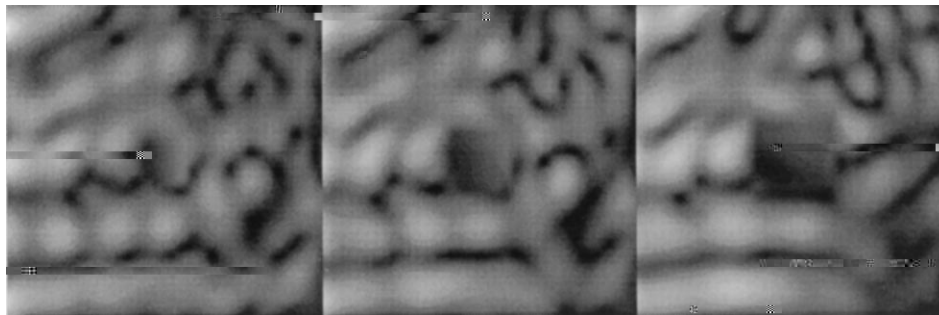
Fig. 9. Grey-scale images of the vertical displacement amplitudes at a vibration frequency of 400 Hz for different size lesions: circle = 4 mm \times 4 mm; diamond = 6 mm \times 6 mm; square = 8 mm \times 8 mm.
